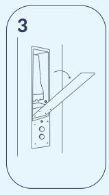
Open service hatch 1. Push the service button until it starts blinking.
