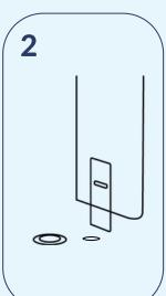
Place a rinse tablet on the floor in front of service hatch 2.
