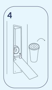
Remove the used filter and dispose of it.
