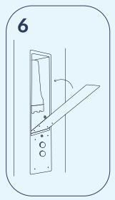
Push the service button to register the filter change. Push the filter container up and close the service hatch.
