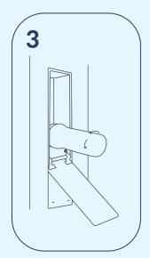
Unscrew the filter container by turning it counterclockwise. Do not use tools.
