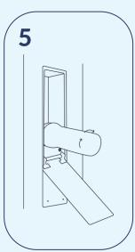
Rinse the filter container under a tap, and insert a new filter. Screw the filter container back in by turning it clockwise. Do not use tools.
